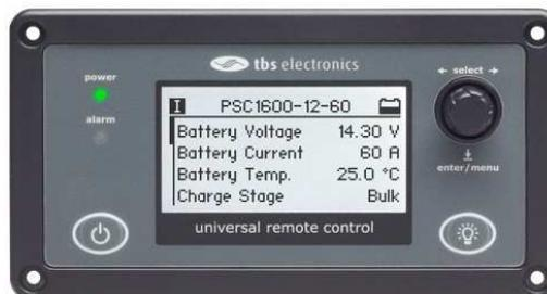
Remote-LCD programmable. 130x70x36mm
